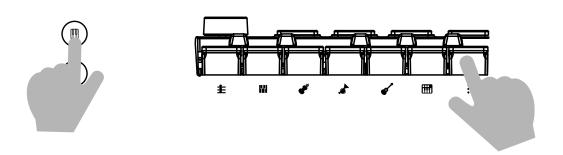
Hold down the  $\bigcirc$  button and press the keys that correspond to the desired sound icons to change the sound of keyboard.
