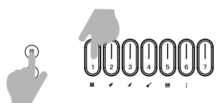
Hold down the button and press the Touch Bar that correspond to the desired sound icons to change the sound of chord trigger mode.
