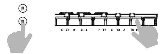
Hold down the button and press the key that correspond to the desired transposition. The blue LED on the pressed key will indicate a successful transposition.
